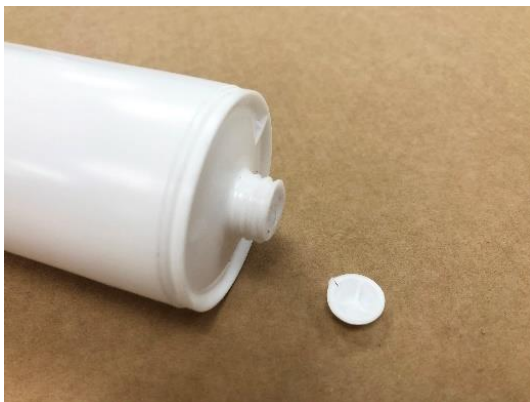
Cut off sealed end of Euro Cartridge
