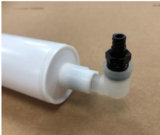
Syringe Transfer Option: Attach adaptors TSD918-3 (Elbow) , TSD931-15 (Female Luer Lock) + empty syringe
