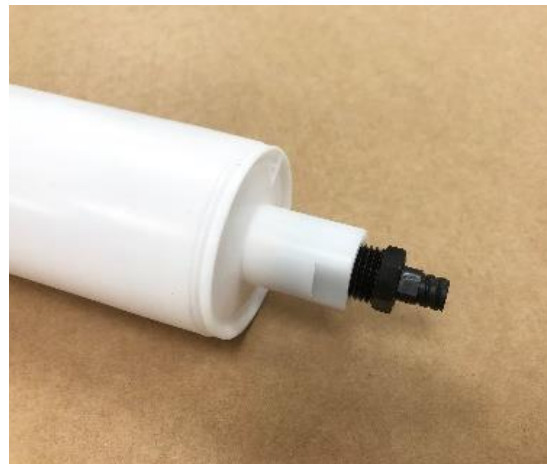
Syringe Transfer Option: Attach adaptor TSD931-15 (female Luer lock) + empty syringe
